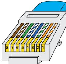
**RJ45 PINOUT T-568B**
